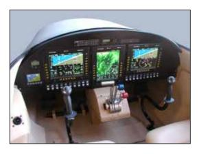
OP Integrated is the latest in the line of Electronic Flight Instrument System (EFIS) and Multi-function Display (MFD) products by Op Technologies. Years of avionics engineering experience have led to this evolution in the Flight Op product line to provide the only truly integrated flight deck solution developed specifically for the experimental aircraft market. OP Integrated combines the Flight Op EFIS
